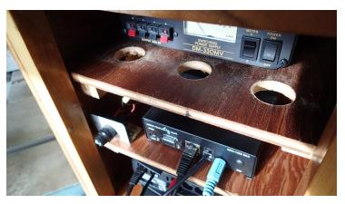
the power supply and radio RRC. Residing under my workbench in the garage, the box had to have cooling and look decent. I built a custom box from plywood with three interior shelves sized for each module, with openings for air flow.
