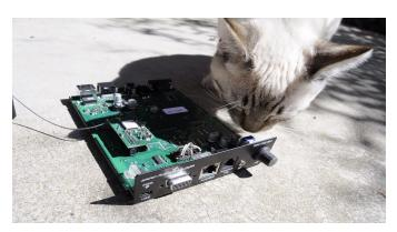
radio transceivers available on the market from ICOM, Kenwood, Yaesu, Elecraft, Alinco and Tentec. Because most Internet Service Providers (ISPs) change your outside internet address, Microbit provides a unique address using their own dynamic DNS service. This allows the control RRC to find your radio anywhere on the internet.
